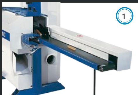
Unloading belt with kicker 1000 x 100 mm / 2000 x 100 mm
