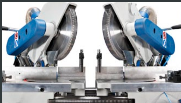
Pneumatic carriage between the two heads for the automatic shifting of the work piece when cutting short pieces. (TR2B I INT)
