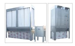
For your growing dust collection needs, look no further than the "FM" series of modular systems! Designed for indoor or outdoor use with hot air re-circulation vents, the FM units are available with motors ranging from 7.5 to 30 HP, motorized shaker units, and noise dampening enclosures. Featuring multiple filter bags made of special woven felt (16 per module), CORAL FM units provide high efficiency at an affordable price.
