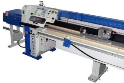
*Automatic push fed saw for optimized cutting and defect removal*
